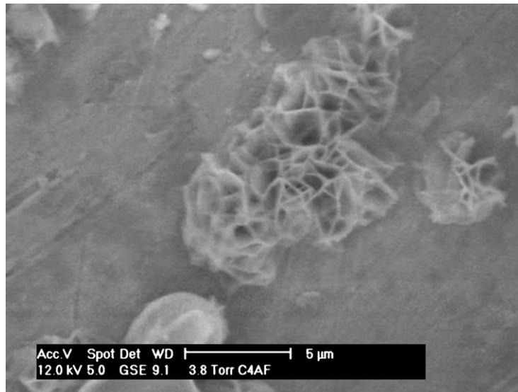
Figure 3 C 4 AF after 13 min hydration. Growth of larger C-A-H plates nucleated on the walls of the steel cup showing inter-connected network.
